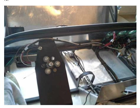
This proto shows the wires at the back of the wiper switch.
